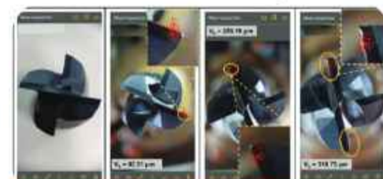
(a) New tool; (b) initial state; (c) intermediate state; (d) worn tool
